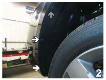
Using a 7MM socket, remove on metric bolt from just forward of the front tire on the edge of the wheel well cover. Set bolt aside to be reinstalled later. Remove two pushpins from the same location. Set pushpins aside to be reinstalled later. Do this to both sides of the vehicle.
