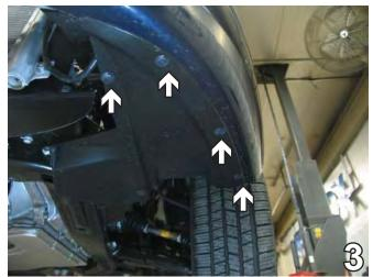
3. Remove four pushpins from the bottom edge of the fascia, just forward of the front tire. Set the pushpins aside to be reinstalled later. Do this to both sides of the vehicle. Pull fascia's upper corners out to the side of the vehicle and straight forward. Set the fascia aside to be reinstalled later.
