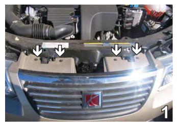
1. Using a 7MM socket, remove four metric bolts from the top side of the fascia. Set the bolts aside to be reinstalled later.
